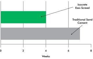
Drying time to receive finishes (BS8203) in good drying conditions (20 $^{\circ}$ C, 50% RH, good ventilation) from removal of the curing polythene sheet.
